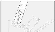
Carefully guide the brake calliper over the mounted brake disc.
